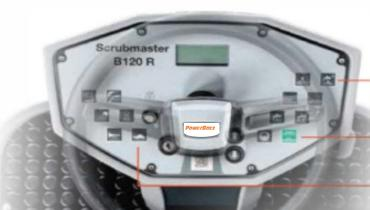
The boost button activates both maximum brush pressure and water flow.
